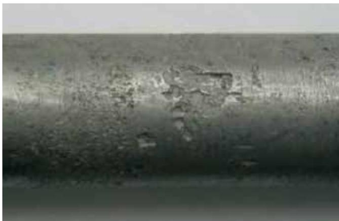
Fig. 4. Stem corrosion due to galvanic corrosion.
