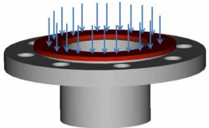
Fig. 6. Gaskets need stress over the entire surface of the gasket.
