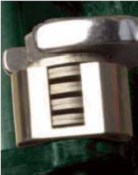
Fig 3. Live Loading Assembly.
