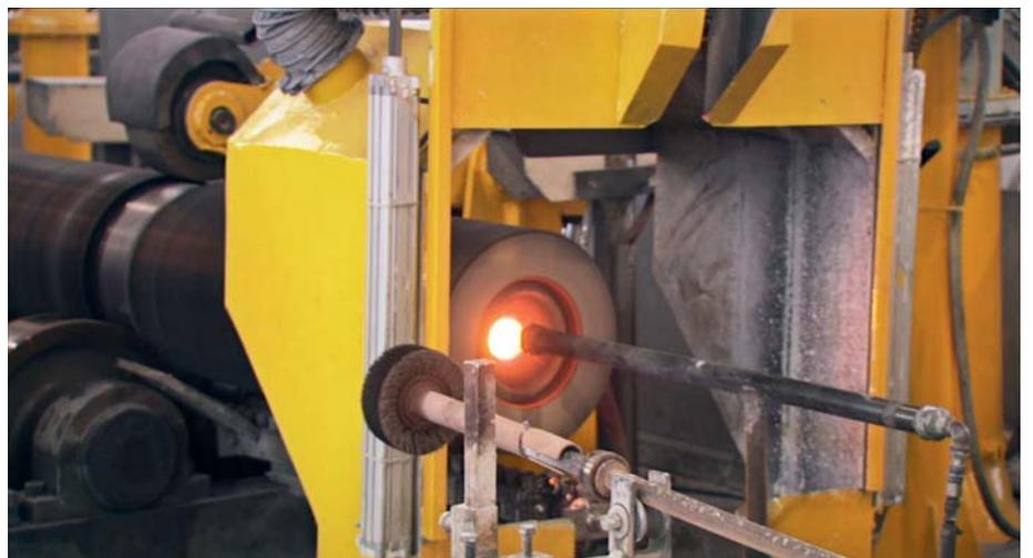
The centrifugal casting production method is one of the core technologies of the Schmidt+Clemens Group.
