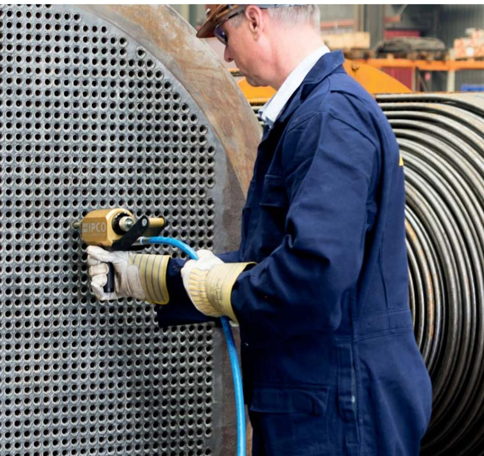
*“The IPCO plug is a product that was especially designed as a solution for tube leakage in shell and tube heat exchangers, a type that is found in almost every part of the heavy industry, including big refineries and chemical plants.”*
