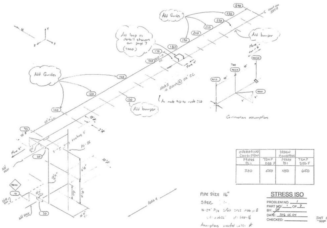
A hand drawn pipe isometric proposes a new design. Here are notes showing movements and clouded directions from the pipe stress engineer.
