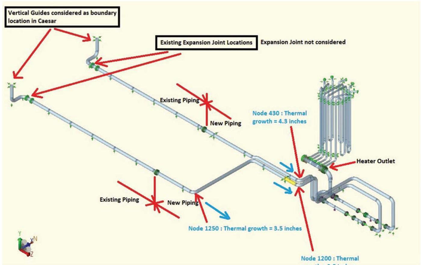
This is a screenshot from the finite element analysis software, Caesar, appended with notes from the designer. Large movements in the piping downstream of furnaces often require expansion joints to safely install. This is to accommodate space-constrained existing facilities.
